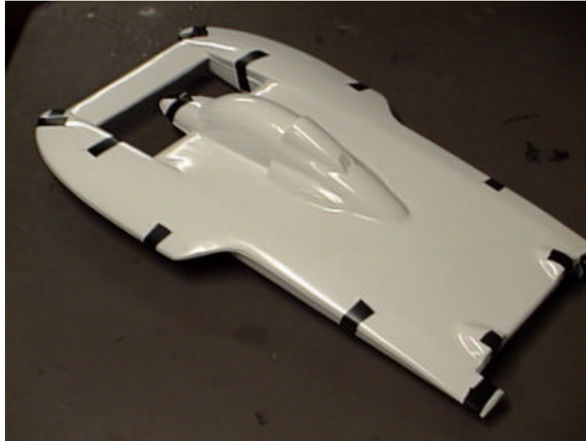
Photo 5 – Hull and Deck Taped Together (Top View)
