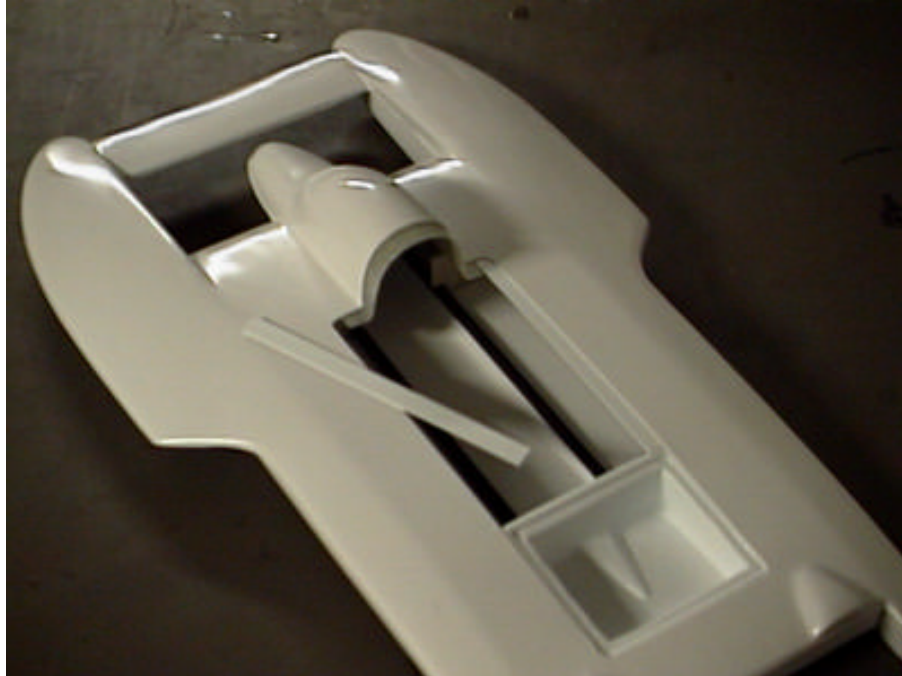
Photo 9 – Radio Box and Ledge Strip Installation
