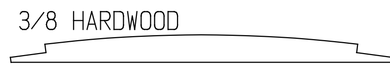
FWD HATCH BRACE 3/8 HARDWOOD
